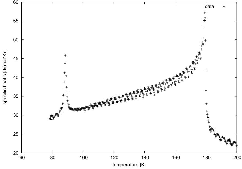
Figure 3: course of specific heat of dysprosium with two phase transition peaks
