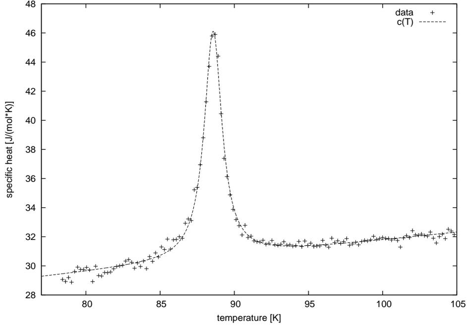
Figure 4: function fitted to phase transition peak of first order
