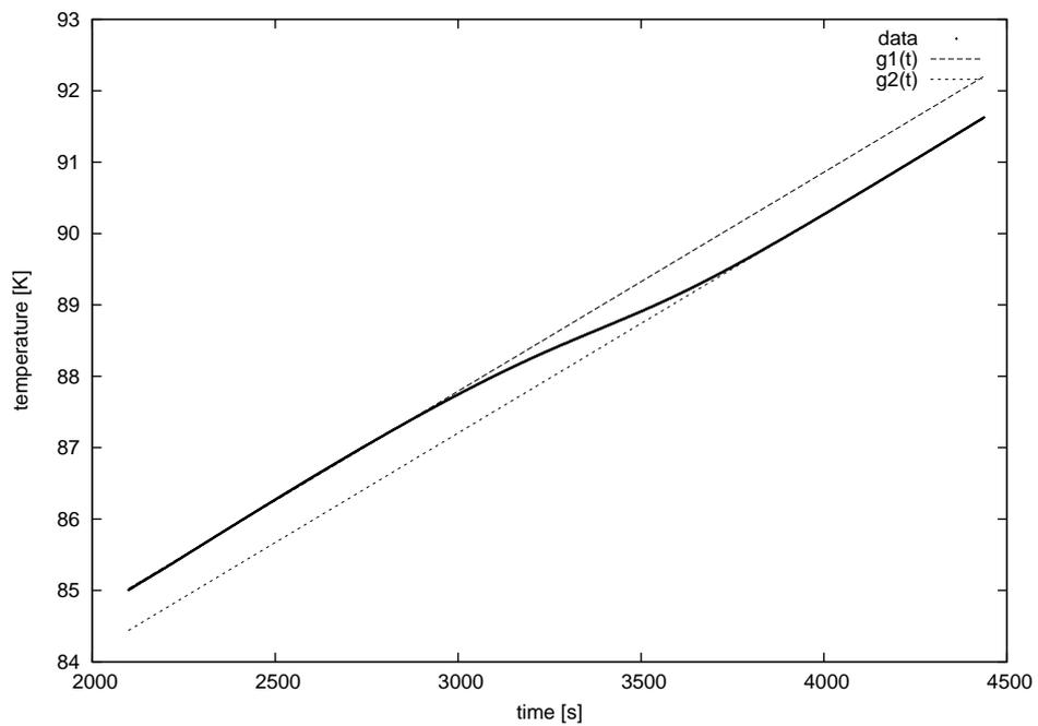
Figure 2: temperature course of dysprosium around the first phase transition with linear fits before and after the transition area
